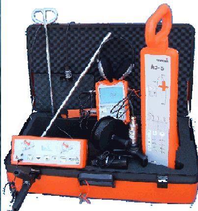
LEAK LOCATION COMBINED WITH PIPE LOCATION
